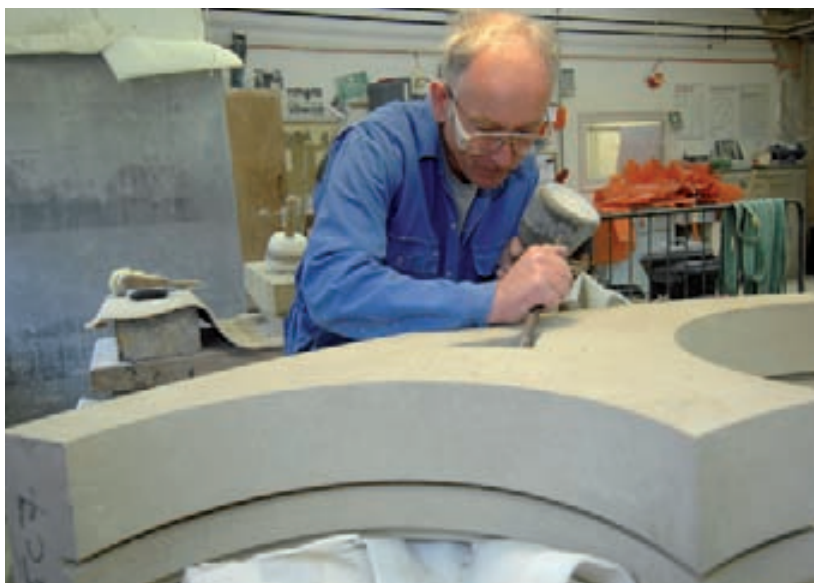
Producing a template for the stone which the sawyers will use.
